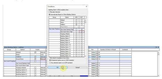
SoftPlan 2022 introduces user-defined conditions to automatically determine when the visibility of a building option should be on or off. By specifying these simple AND/OR conditions, you can control the visibility of complex building option configurations without the need to manually set the visibility for each related building option every time.
